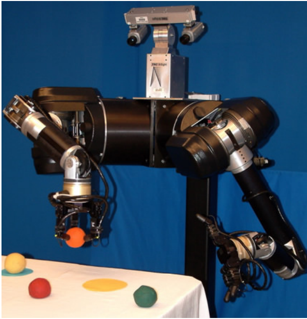
Figure 1: Dexter, consisting of two seven-degree-of-freedom manipulators, integrated three-fingered hands with high-resolution tactile sensors, and a four-degree-of-freedom stereo camera head. Not shown are several webcams and a glove-like input device that enable remote operation over the Internet.
